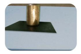
As shown in the epoxy picture, the falling object (weighing 3 kg, dropped from a 3 m height, with a strike point radius of 0.5 mm and a cone angle of 60 degrees) penetrates completely the laminate and sticks into it.
